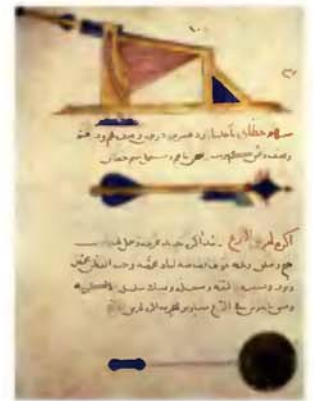
Cannon with adjustable mounting from a 14 th -century Manual on Armoury by Ibn Aranbugha al-Zardkash.
